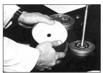
FIGURE 8 - ASSEMBLY OF DESICCANT CARTRIDGE
