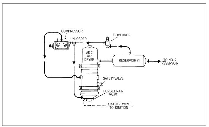
FIGURE 18 - TYPICAL INSTALLATION FOR THE AD-2
